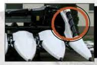
ROTARY END DIVIDER Using the rotary end divider when the corn is tilted, will considerably reduce the losses.
